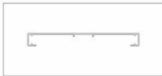
25.2X270 Silent mouthpiece wall thickness: 2.7 mm Applicable wall thickness: 228mm-247mm
